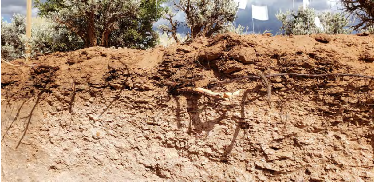
Photo 8. NR-3 test pit showing platy structure and highest root density within top 8 in of silt. Roots extend horizontally above underlying layer of silt and clay with increased caliche cementation.
