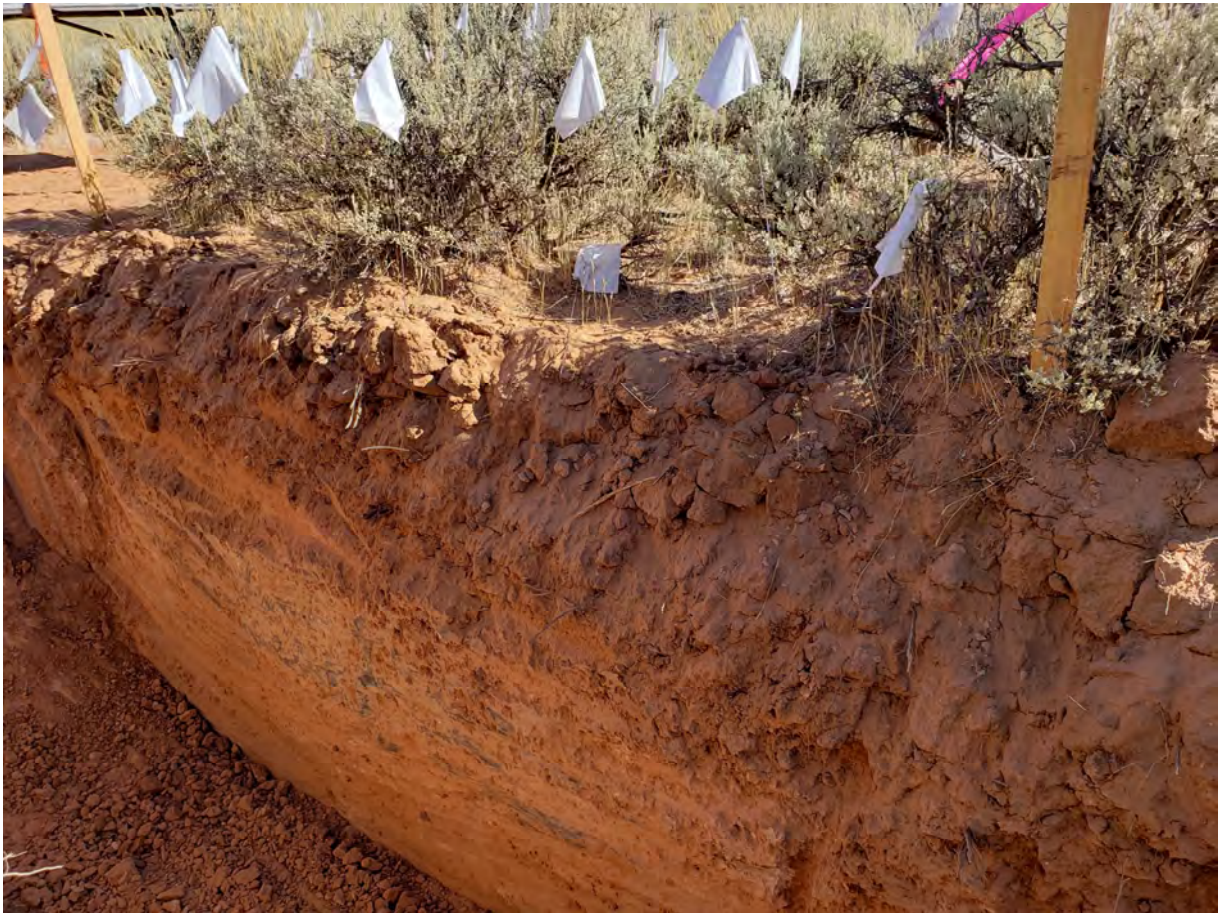
Photo 2. NR-1 test pit profile (4 ft depth) showing highest root density within upper loose silt and increasing caliche cementation with depth.
