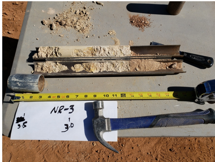
Photo E-1-4. NRB-3 alluvium-weathered sandstone contact.
