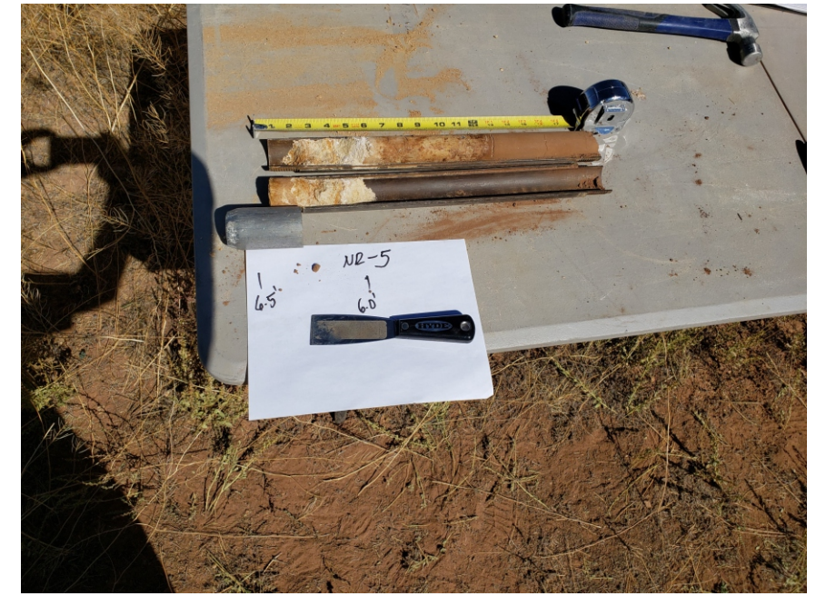
Photo E-1-6. NRB-5 alluvium-weathered sandstone contact.
