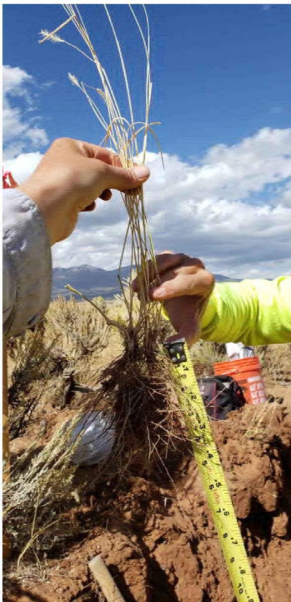
Photo 5. Measuring grass root length at NR-2 test pit.
