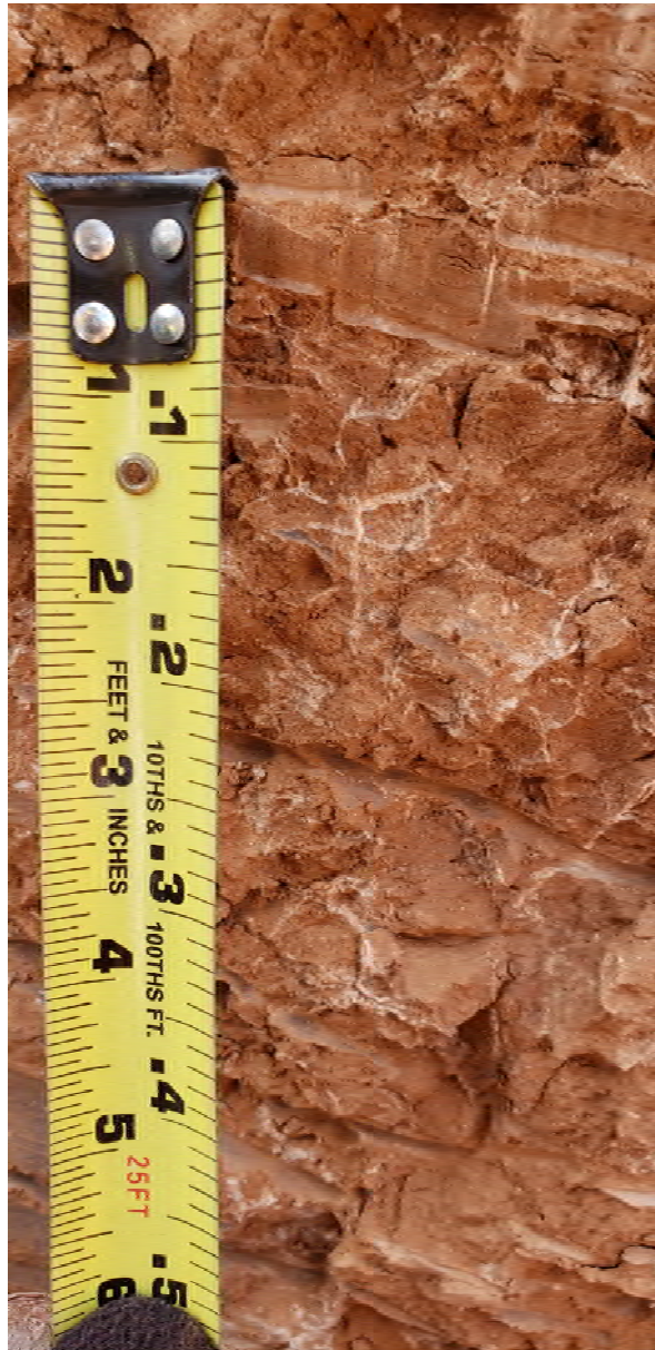
Photo 6. Measuring caliche root casts at 2.5 ft depth in NR-2 test pit.
