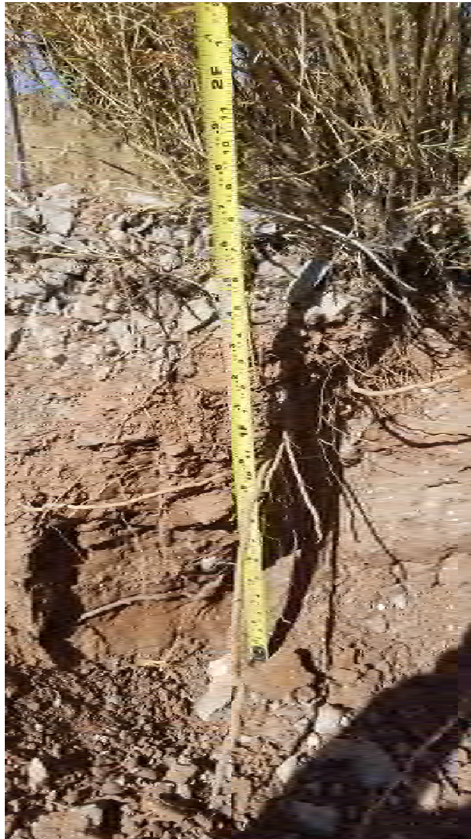
Photo 22. Rubber rabbitbrush root profile at LT-TP1 test pit with highest root density within top 0.75 ft and taproots extending to 1.75 ft depth.
