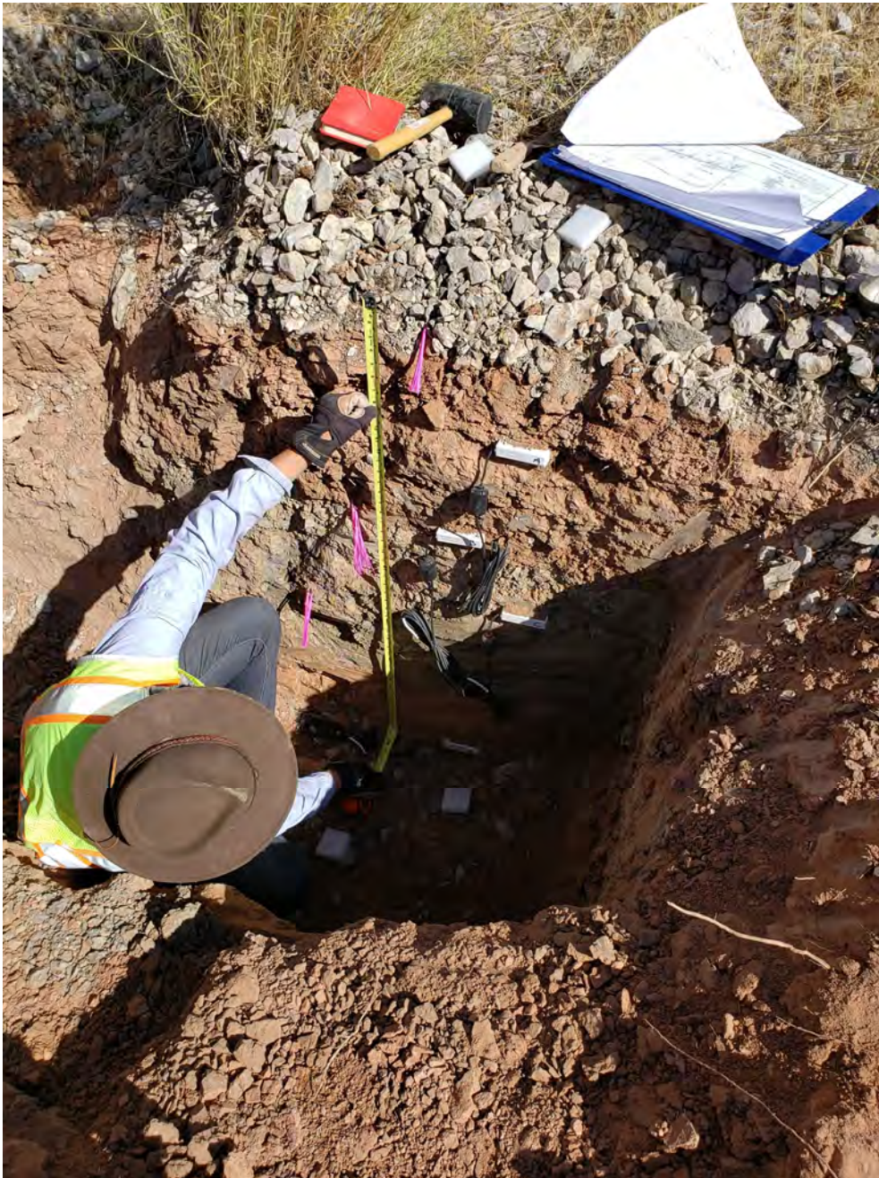
Photo 25. Soil moisture sensor installation at LT-TP2 test pit showing four sensors in series. The shallow sensor was installed in the upper silt layer within the highest density root zone. The intermediate sensors were installed within the platy structured clay layer and the deep sensor was installed in clay below the EZD near the base of the 3.9 ft excavation.
